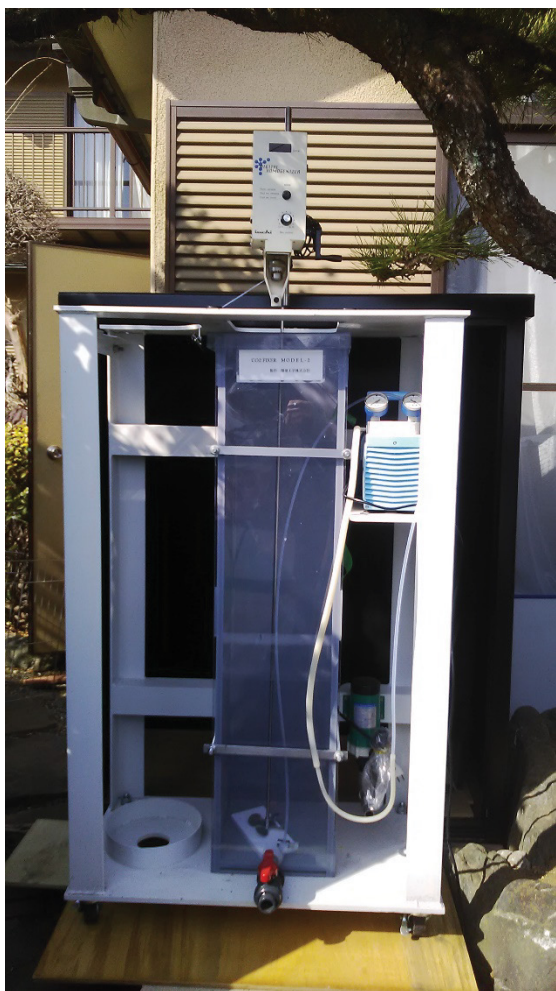
Figure 3: Photo of CO 2 fixation process. The reaction tank (26 × 28 × 120 cm) was settled in the white frame (43 × 80 × 125 cm), and the axle with a screw propeller was driven by a motor on the top of the frame. Air pump (Multi Dry Pump Suction-Discharge Convertible Type, MP-30) was purchased from As One (Tokyo, Japan).
