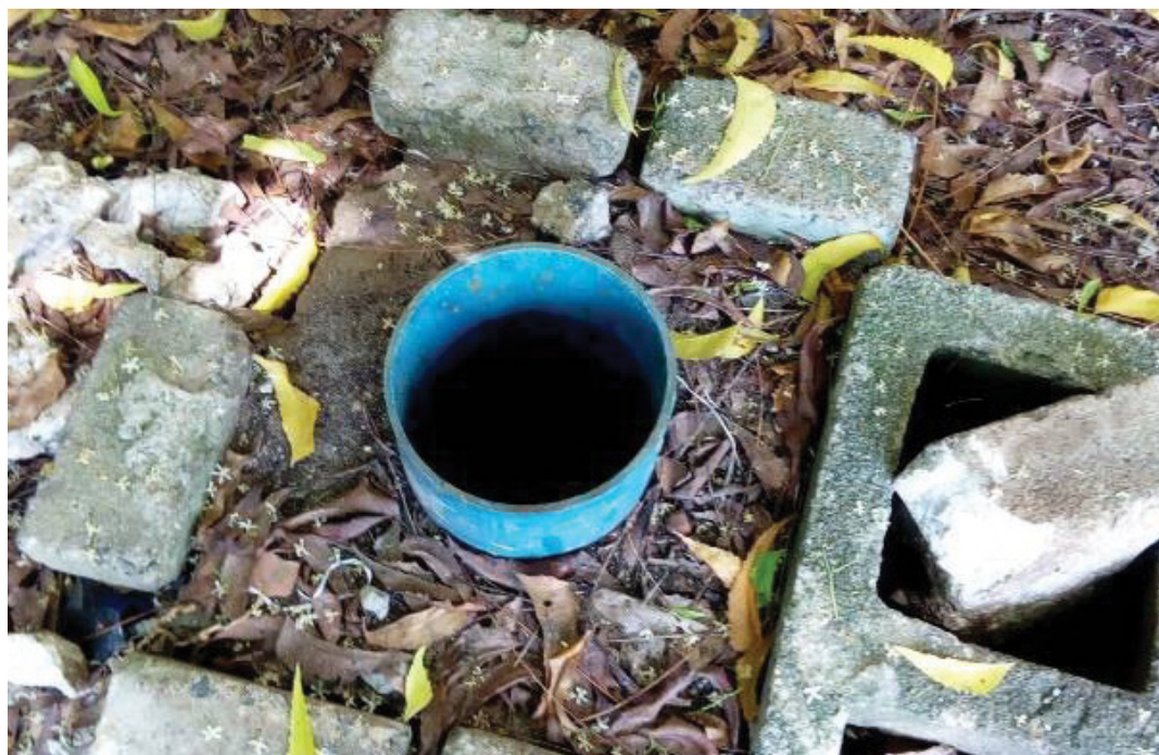
Figure 2: The 200 feet monitoring borehole at the front of the department of physical and chemical oceanography (~140 m from the NIOMR Jetty).
