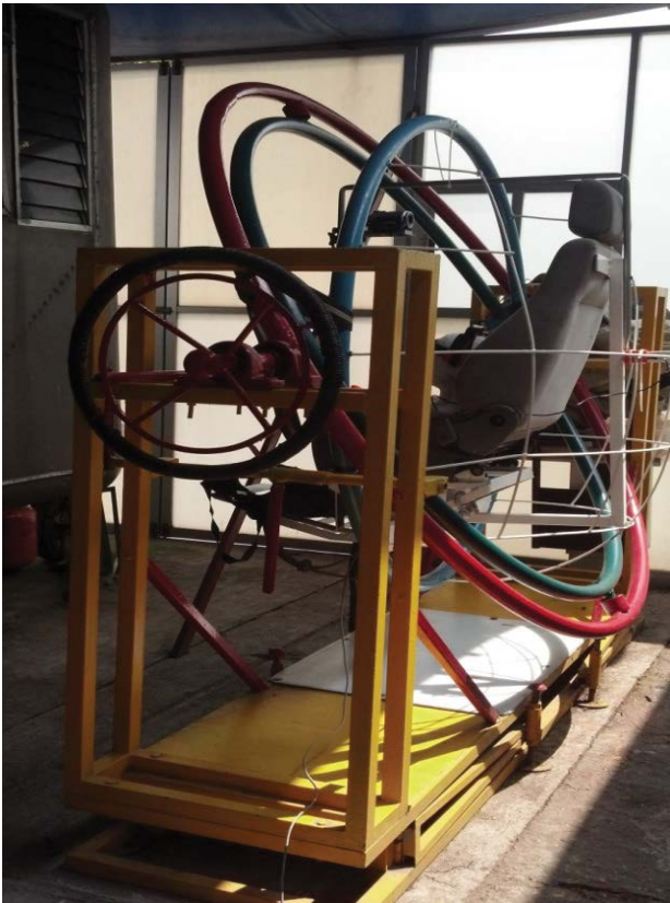
Figure 2: Mounting of human gyroscope to capture movements.
